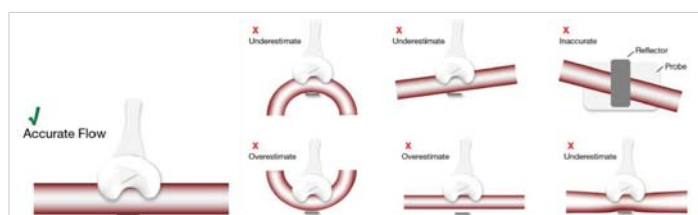
Figure 15: Correct placement of the probe vs. examples of inaccurate placement of the probe (images provided by Medistim®).
